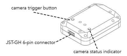
The LED camera status indicator mimics the LED signals on RedEdge-MX. The signal types are outlined in the Sensor Firmware Guide. The camera trigger button will command a capture on the RedEdge-MX. This is useful for capturing a preflight image of the calibration panel.
