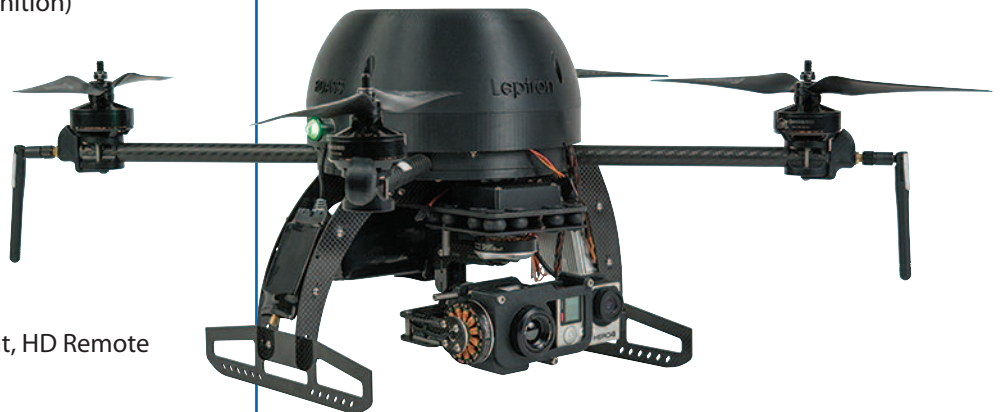
Leptron RDASS HD with optional Stabilized Dual-Camera setup using FLIR VUE Pro and GoPro Hero4 cameras, and optional Navigation Lights
